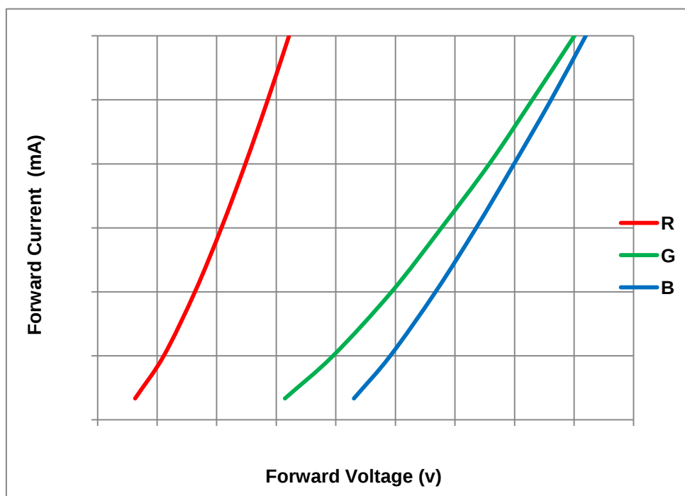
Fig 1-6 Forward Voltage Vs. Forward Current 伏安特性曲线
